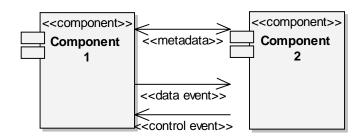
FIGURE 3. A component with metadata and data events, and control events
